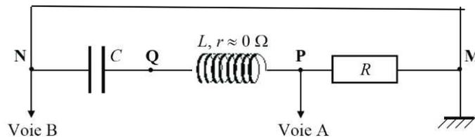
Figure 3. RLC series circuit
